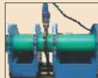
**Alignment:** The two ends of pipes to be joined should be checked for alignment and matching. The gap between two ends must not exceed 0.5 mm at any point.
