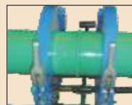
**Apply Pressure:** Press the pipe ends to be joined against the heating element with the required force until the entire circumference of both the joining faces rests completely against it and a bead is formed. Reduce the equalization pressure to zero.
