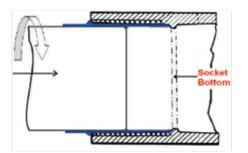
3. Assemble the pipe and fitting while the surface is wet. Rotate the pipe up to ¼ turn, and push in to the socket until it reaches to the bottom of the socket.
