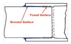
4. The interference fit design allows the pipe and fitting to fuse together. The bond is created in the loose section of the joint. Joint strength develops as cement dries.
