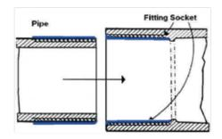
2. Apply a layer of cement in the fitting socket, and a layer of cement on the pipe. Sufficient cement should be applied for proper gap filling.
