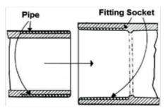
1. Area of pipe & fitting to be soften by solvent cement
