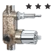
F4010105 Concealed body for turn type single lever concealed diverter system consisting of 35 mm cartridge with button Assembly, Cartridge Sleeve (but without operating lever, wall flange and tip ton knob) Water saving 40%
